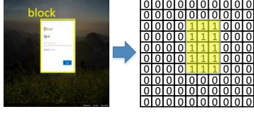
Figure 8: Pixel-matrix representation of block layer in the AWL input channel, assuming that the shape is 10 \times 10 .
